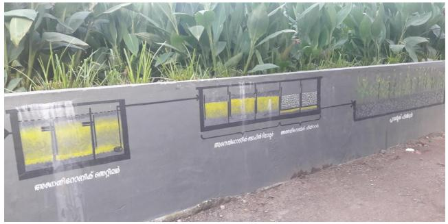
Fig.18.20 Planted gravel filter in DEWATS system in the slum area at Chathanad
