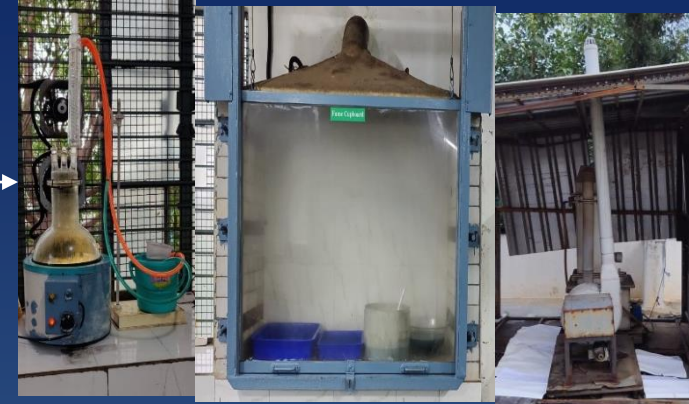
Glass Plant For Metal Extraction By Leaching attached to air Pollution control unit at the exhaust
