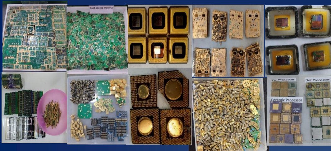
Sources of Gold Plated E-Waste (Network boards, Processors, Components, Connector pins etc)
