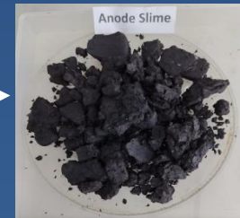
Anode Slime recovery by electrolysis for precious metal by Smelting of PCBs using C-Met Technology
