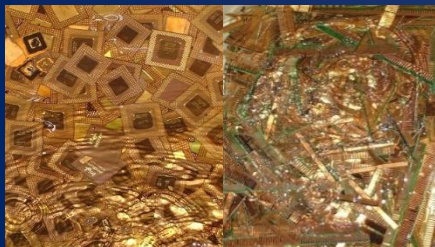
Selective Recovery of Gold from Segregated Gold Plated E-Waste using Selective Aqueous Strippers for Apparent gold plated areas only.
