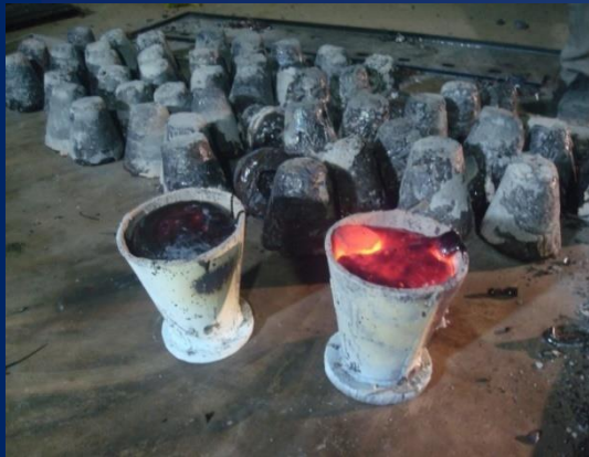
Metal & slag collection in MS Ladle
