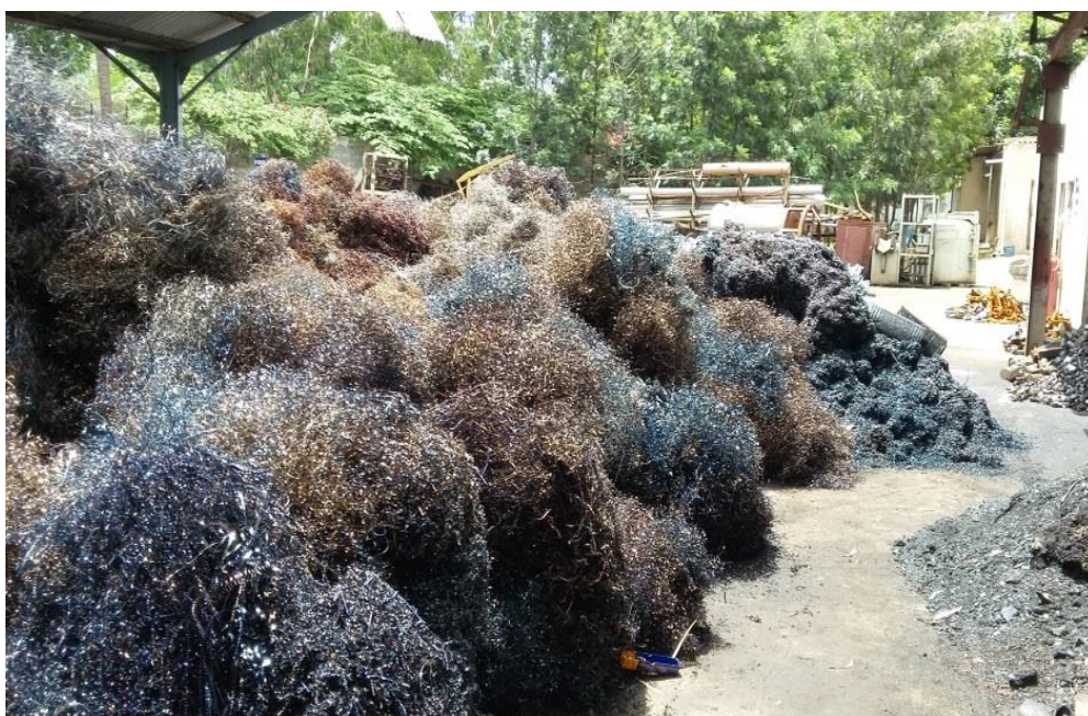
Figure 3.2 Waste from lathe industries
