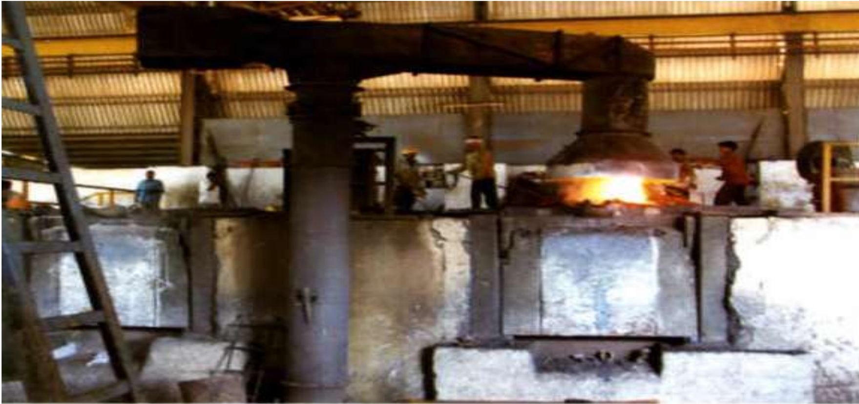
Swivel arrangement with underground ducting
